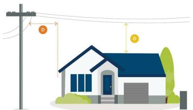
Please ensure that structures, such as garages and extensions to houses, remain well clear of overhead lines.
