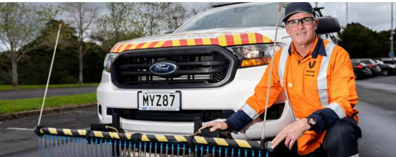
Our Field Service Provider Omexom uses a truck-mounted gas leak detection system known to 'smell' minor gas leaks by simply driving down the street at normal speed, with GPS technology marking the exact location of any leaks detected. This enables us to find and fix leaks faster, reducing carbon emissions and improving the safety of the public and environment.
