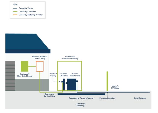
Option 2: Vector installs its own substation (transformer and LV frame in an outdoor enclosure) inside the customer's property.
