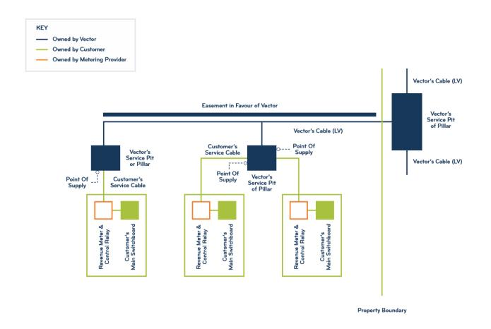
Note: Vector accepts reticulating inside right of ways provided that the customer agrees to grant an easement in favour of Vector to protect the equipment and allow Vector to operate and maintain the equipment. Vector will keep / maintain records of this equipment and the easement protecting it.
