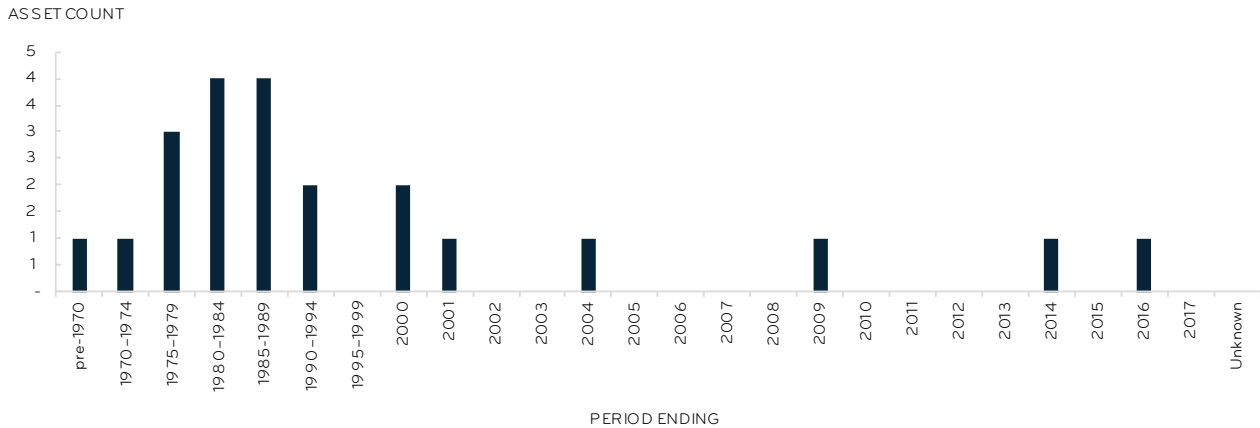
Figure 4-7 Age profile of the corrosion protection equipment
