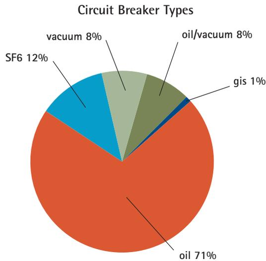
Figure 7.2 Subtransmission circuit breaker by type
