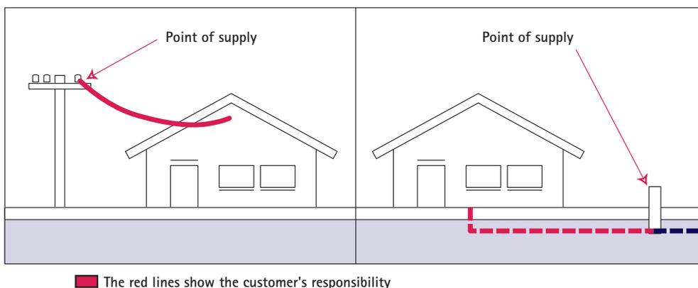
Figure 4.2 Typical customer connection point
