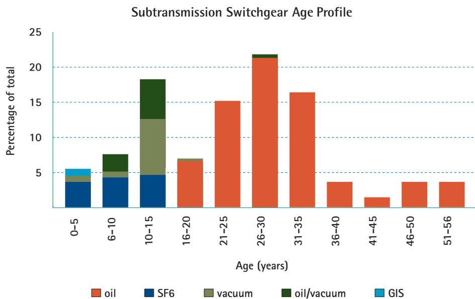
Figure 7.3 Subtransmission switchgear age profile
