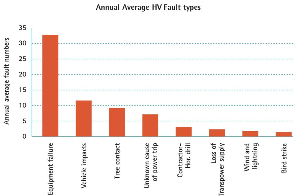
Figure 3.3 Typical HV fault types
