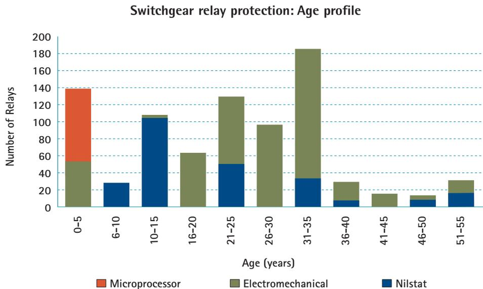
Figure 7.8 Age profile of Switchgear relay
