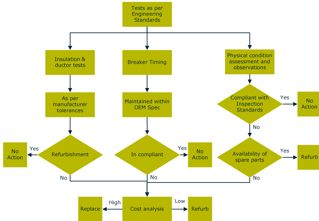
Figure 6-13 : Zone substation circuit breaker replacement decision chart
