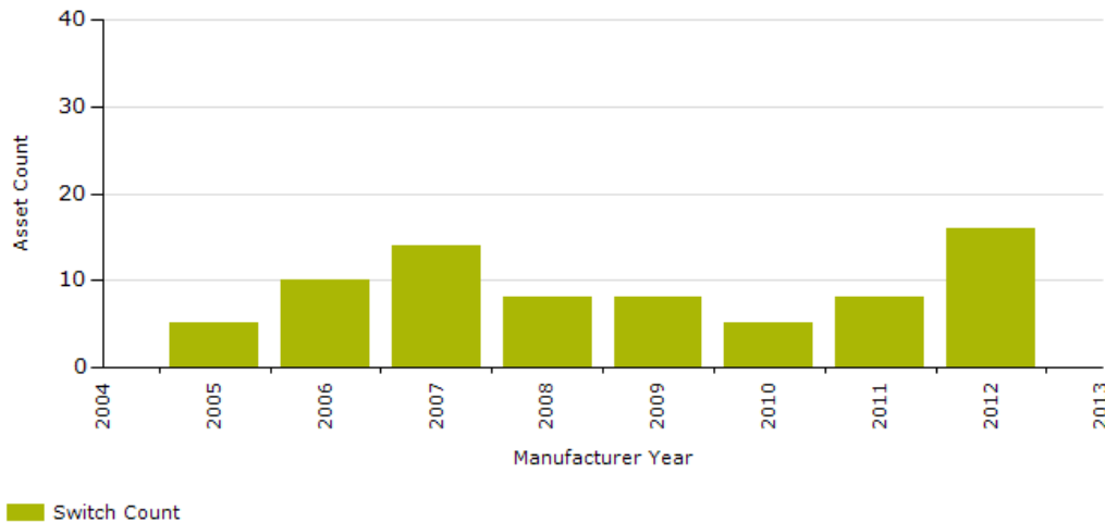
Figure 6-23 : SCADA ethernet switches age profile - Northern
