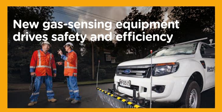
A vehicle equipped with a 'moustache' to sniff out gas leaks across Vector's vast pipeline network is delivering improvements in safety and reliability and lowering costs across our 7,245km gas distribution network.
