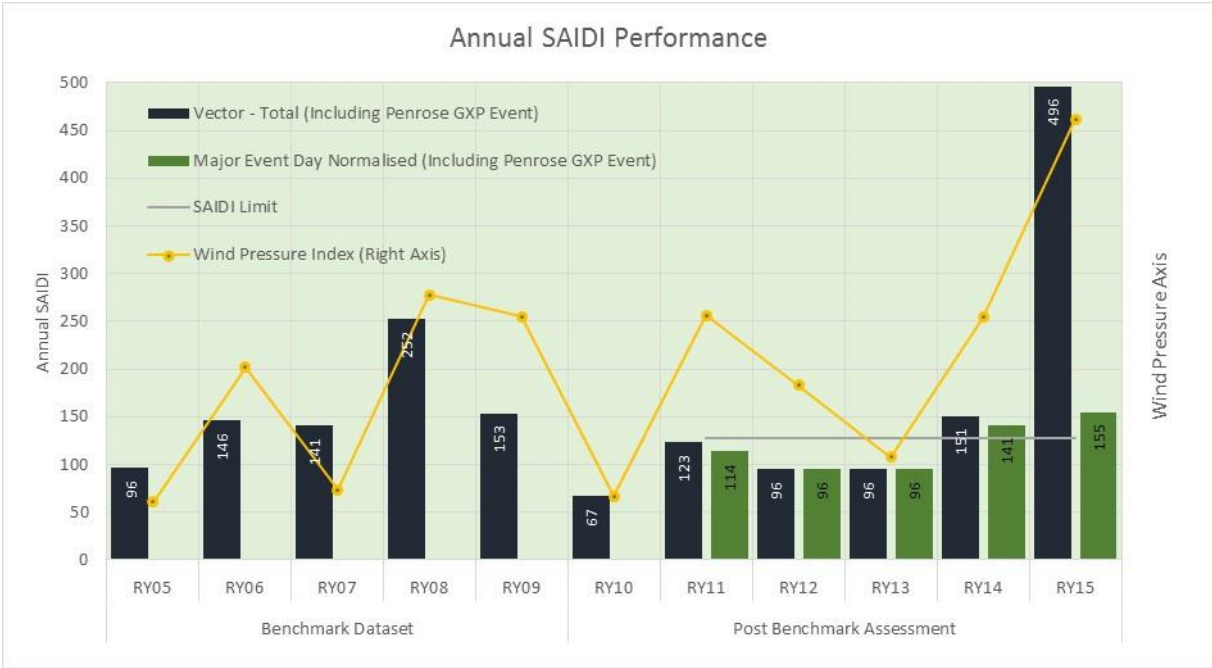
Figure 8 – Relationship between wind pressure for wind speeds >60kph, and network SAIDI performance
